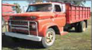
1966 Chevy C-60 truck, 366 eng., 5 & 2 spd. trans., good rubber, grain box 15' 5", 40" side, metal floor, rollover tarp, 59,531 miles
